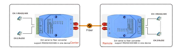
Case two: DIP1=ON, channel cross, the RS422/485 of channel 1 of one device is connected to the RS232 of channel 2 of another device; the RS232 of channel 2 of device is connected to the RS422/485 of channel 1 of another device.
