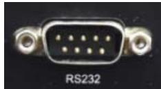
**DB9 is DTE mode, it multiplexed with access terminal, they can not be used at the same time.**
