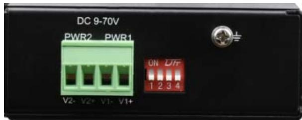
**Factory reset:** dial up the 4<sup>th</sup> pin before the device is powered on, **and then dial down the dial after power on, the device will power off and restart, and the running indicator light will flash again.**
