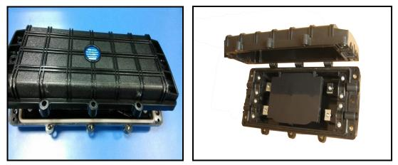
TELESYSTEM's in-line fiber splice closures are compliant with IEC 1073-1 and YD/T814.1. The closures are made of tough anti-corrosive Polycarbonate that makes the closures ideal for aerial, cable duct, direct burial and well applications.
