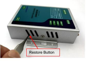
To use tweezers press the button at **5 seconds**. And see the LINK LED will went out and then on. It's mean the restore is success.
